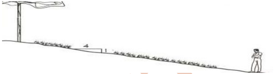
Figure 2.12: Illustration of a 4:1 Slope Ratio
